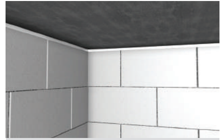
Top of wall construction joint
