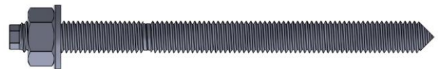
Example of threaded rod with hex drive, depth mark and chisel point for installation with spin-in capsules
