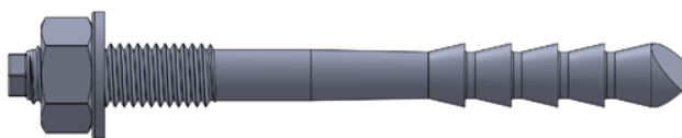
Example of torque controlled anchor rod, tapered cones transfer loads through resin in cracked concrete.
